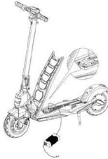
Connect charger to the charging port (B).
